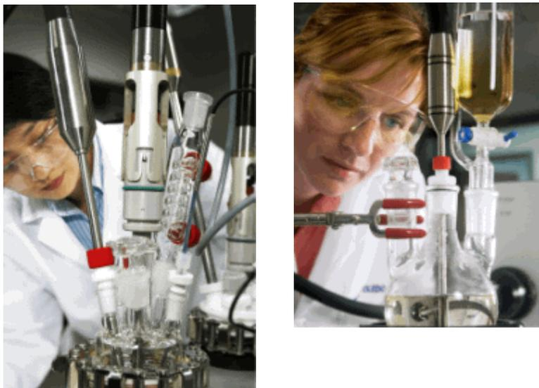
**Figure 4-7 DS FiberConduit with adapter in common reaction vessels**
