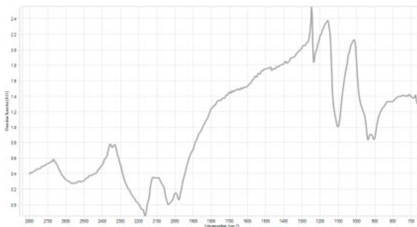
Figure 4-17 Abnormal peaks from changed sensor without new background
