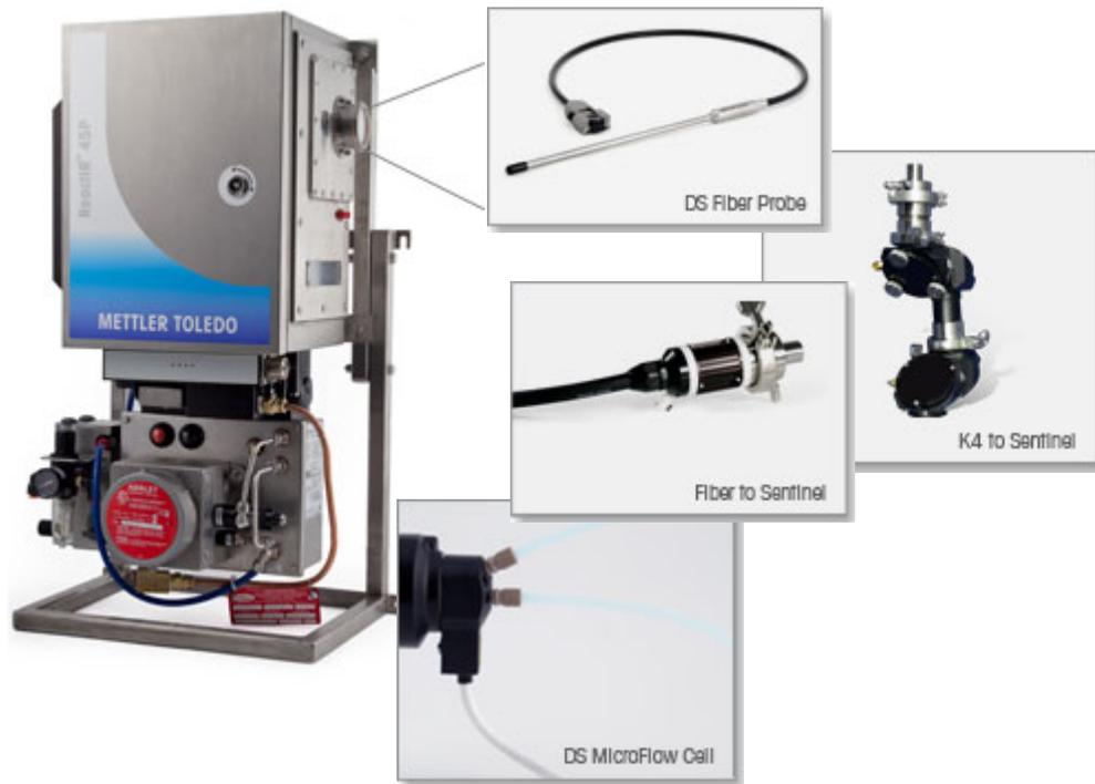
**Figure 2-4 ReactIR 45P HL base unit with representative sampling technologies**
